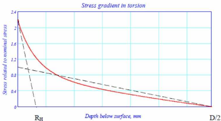
Fig 19 Torsional SCF in the crankpin fillet as a function of depth. The corresponding SCF for the journal fillet can be found by replacing R_H with R_G and D with D_G
